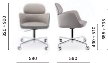
695 Upholstered armchair, die-cast four-star aluminium base with castors, adjustable in height
