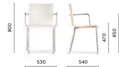
2444 * Armchair, plywood shell upholstered front side, steel tube frame
