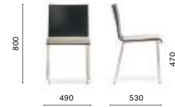
2413/A * Side chair, plywood shell, upholstered seat, steel tube frame
