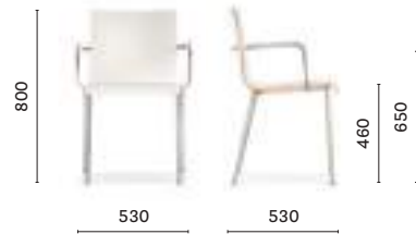
2416 Armchair, laminate shell, steel tube frame
