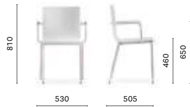
2415 Side chair, laminate shell, steel tube frame
