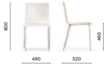
2416 Armchair, laminate shell, steel tube frame
