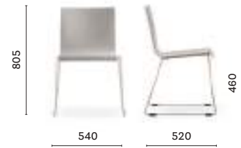
2409 Side chair, technopolymer shell, steel rod sled frame
